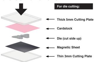
Use this combination for foam, card, glitter card, acetate, shrink, plastic, balsa wood, and foil.
