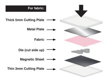
Use this combination for leather, cotton, silk and craft metal. The thickness of the fabric will determine the number of layers which will cut in one pass.
